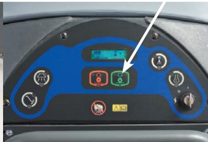
Single touch button control sets proper operation of all functions. Simplifies training and consistent use by all operators.
