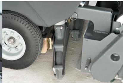
Dual laminar flow vac shoes allow for more efficient recovery of solution.
