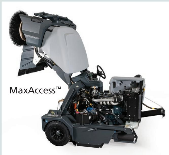
MaxAccess™ interlocking compartments allow for industry-best accessibility of critical components to expedite service and repair.
