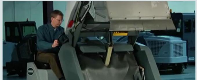
The hopper's safety bar control is located in the cab, maximizing the likelihood of operator use and improving safety.
