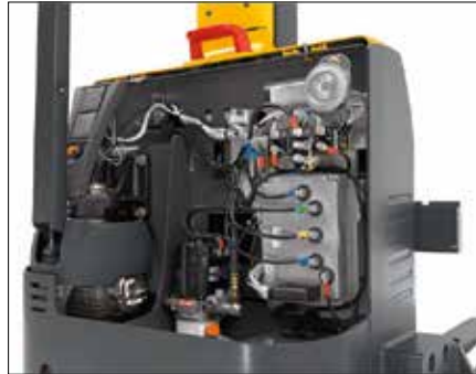
Sealed AC motor, controllers and connectors
