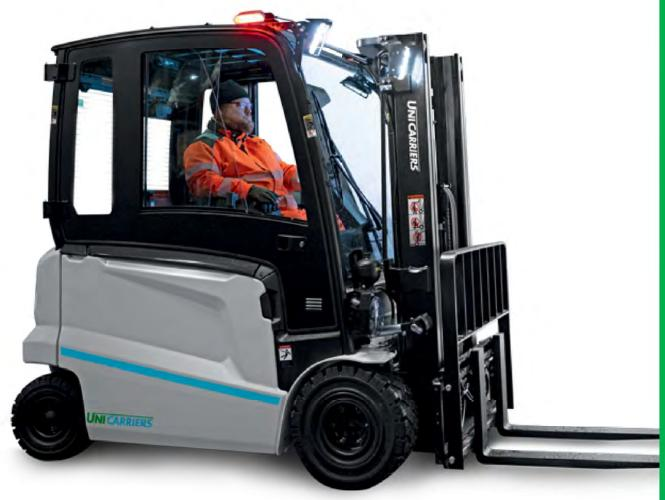
Electric Pneumatic Tire Lift Truck
