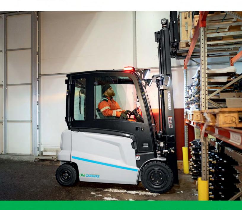
Built for maximum operator comfort, the ergonomically-designed MX2 cabin features a quiet work environment. The electric platform limits noise, increases ease of drive and ultimately eliminates CO<sub>2</sub> emissions.
