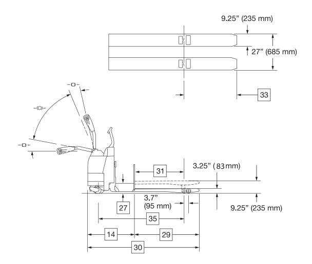
With the handle vertical, add an extra 3/4" to overall truck length. With the handle vertical and rotated 90°, add an extra 2" to overall truck length.
